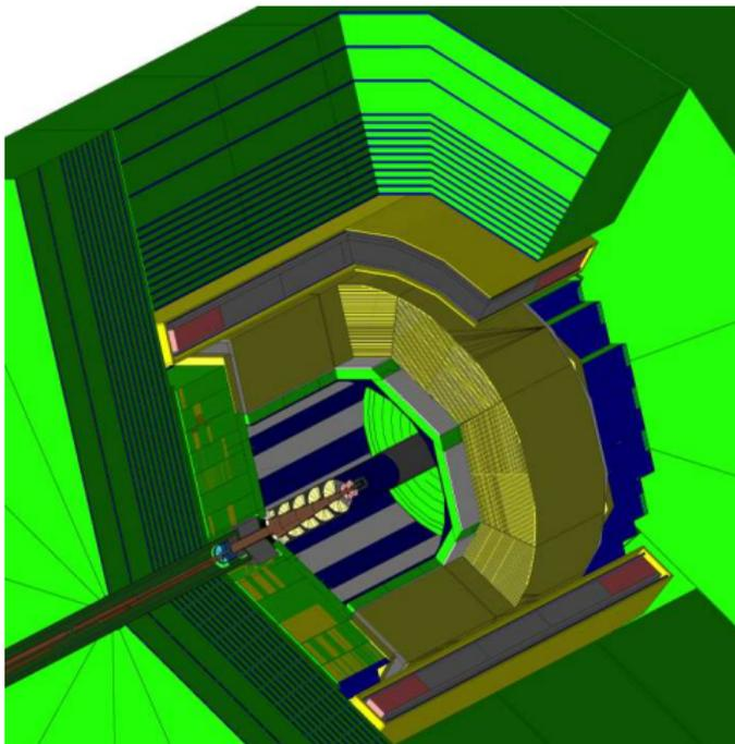
Very detailed implementation of the detector in the full GEANT4 simulation
