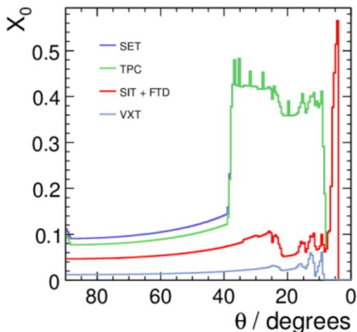
ILD tracking material budget (incl. cabling, cooling, support)
