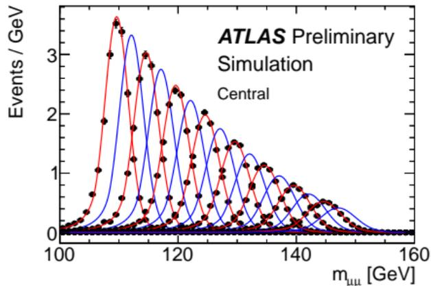
Signal described by convolution of Crystal Ball + Gaussian functions
