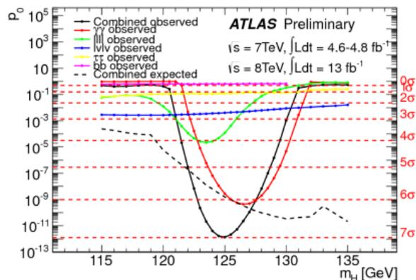
The local probability  $p_0$  for a background-only experiment to be more signal-like than the observation as a function of  $m_H$  for various individual channels
