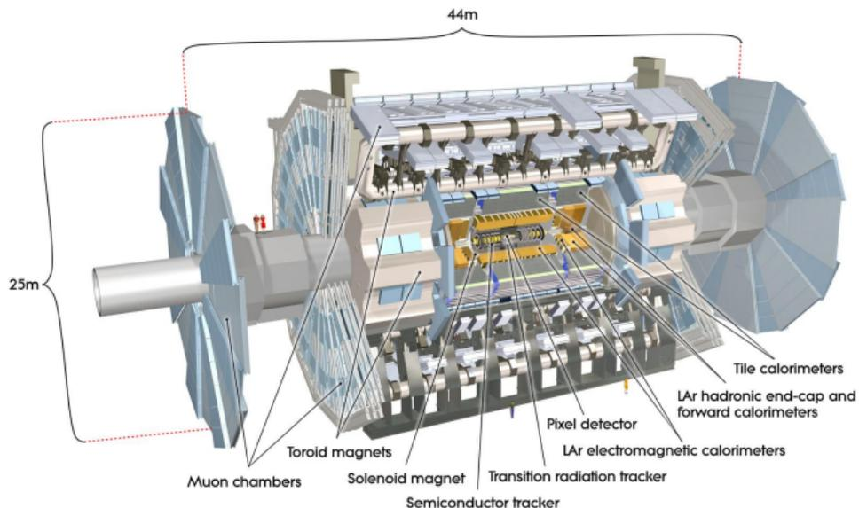
**Magnets:** 2T solenoid 3 air-core toroids
